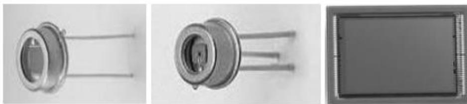
Fig 3. Pin Photo Diode, Avalanche Photodiode and Image Sensor
